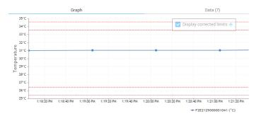
Figure 125. High and low limits corrected for drift and uncertainty
