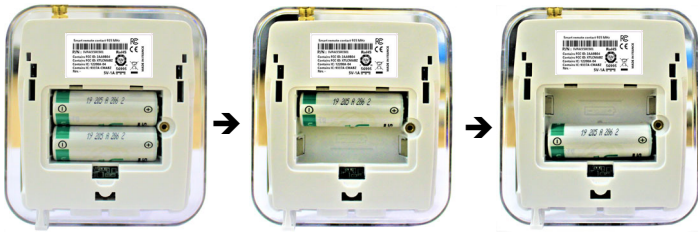
Figure 76. Replace one battery after the other (and/or keep AC power on)
