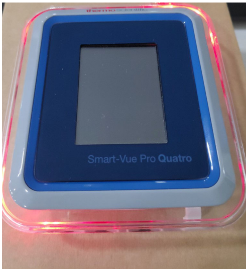
Figure 67. Data logger with alarm condition indicated by red LED
