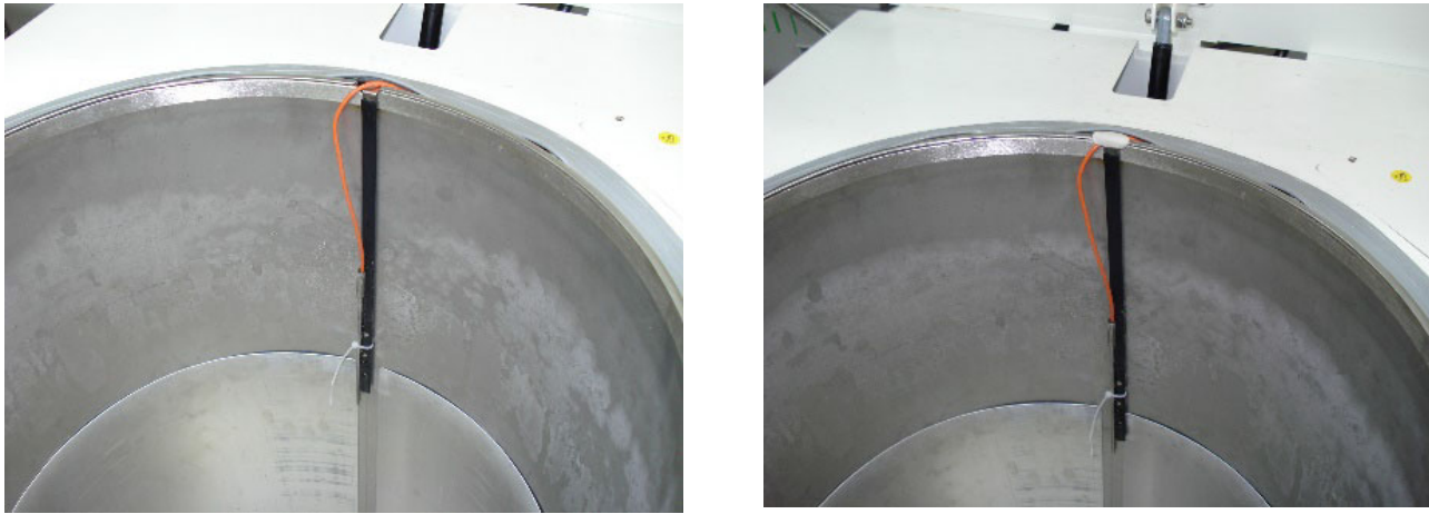
Figure 22. Pt100 (-200 °C to + 50 °C) for nitrogen/cryogenic tank
