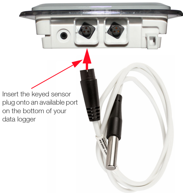
Figure 24. Smart-Vue Pro Duo/Quatro data logger with external digital sensor
