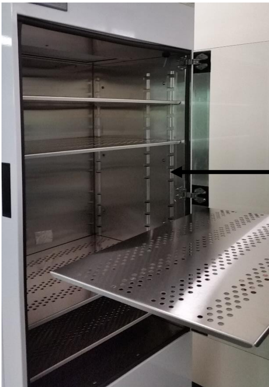
Figure 8: Removing shelf for cleaning and adjustment.
