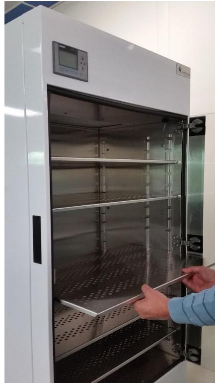
Figure 7: Sliding shelf forward for loading and payload access.
